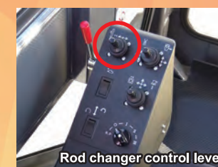
Rod changer control lever
